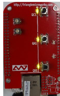
IEC 61850 Stack Implemented on TI Sitara™ AM335x ARM® Development Board
